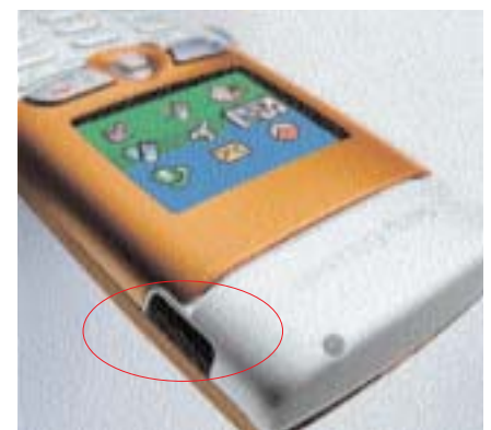
Sony Ericsson T310 is a popular IrDA enabled mobile phone. The black rectangle seen here is the infra-red port
